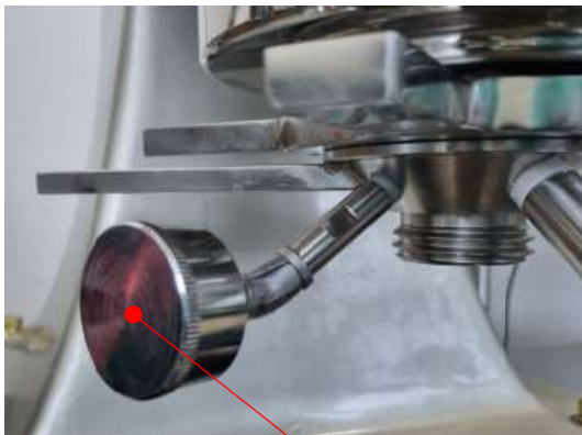
Grease cup: Lubricating grease injection device when bowl rotates
